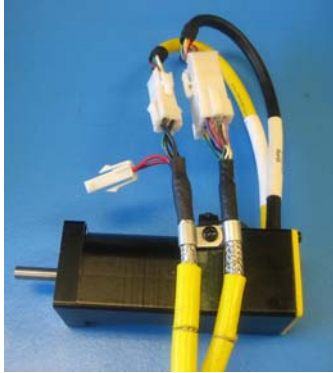
“P” clip attached directly to motor
